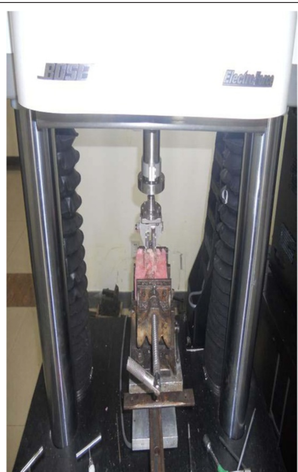
Figure 6 Device used for maximum pullout strength test.
