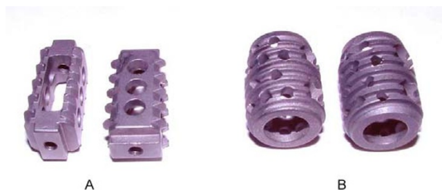
Figure 1 A. The rectangular cages (Corin). It has wedge shape with larger cranio-caudal diameter in front. The teeth are on the cranio-caudal surfaces. There is a large central cavity which can be filled with bone graft. The cages are designed to be inserted with smaller diameter into the disc space, and then rotated by 90° to orient its long diameter cranio-caudally and to engage the teeth into the endplate. B. The Cylindrical cages (BAK).
